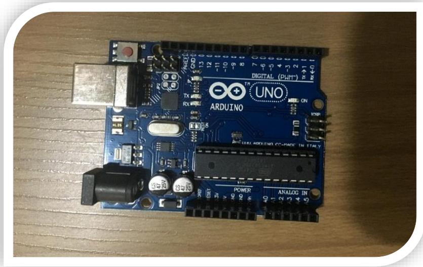
Figura 1: Chip ARDUINO UNO R3
