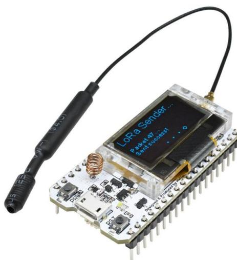
**Figura 5:** Placa WiFi LoRa 32 - ESP32 / LoRa / Display OLED
